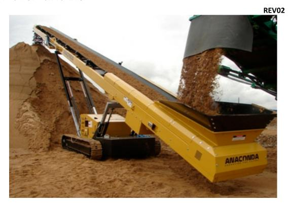
The TR60 is a track mobile high capacity stockpiling conveyor, which is strong and economical to run. The TR60 is versatile and can be used on its own or with other screening plants. Its portability allows it to work in confined spaces and also where heavier conveyors would find it impossible to manoeuvre. The TR60 consists of a track base, feedboot, conveyor, powerunit and has a pendant remote control system.
